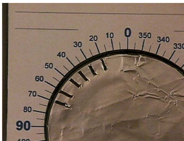
Fig. 2. An example of an Al foil covered collecting disc. In this example, six strips of Al foil were cut at 20°, 30°, 40°, 50°, 60° and 70° for Py–GC–MS analysis. The width of the Al strips is 1 mm.
